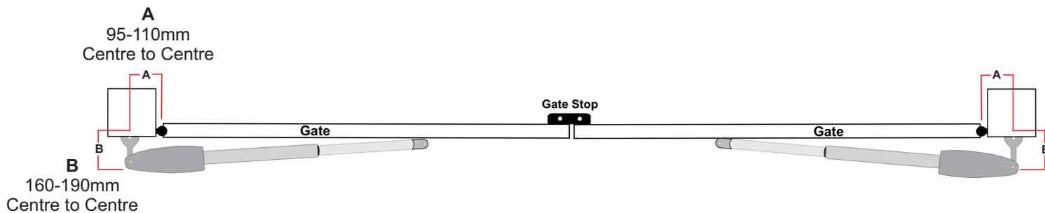
**Gates Closed in a Pull to Open Installation**
